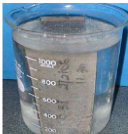
After 1500 hours Mild steel immersed in sea water with 700ppm of Vapro VCI-844L.
